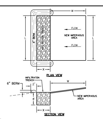
L = LENGTH OF NEW IMPERVIOUS SURFACE (FT) = LENGTH OF INFILTRATION TRENCH
