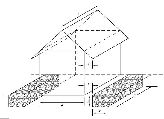
**KEY** L = LENGTH OF STRUCTURE = LENGTH OF SEEPAGE TRENCH (FT.)
